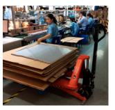
The manual highlifter needs very low power for the pump function and has foot protection and neutral position.
